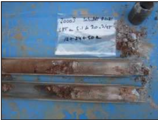
Foto 3: Sondeig S-1, SPT a 3,0 metres.
