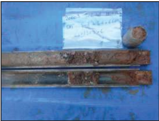
Foto 22: Sondeig S-3, SPT a 6,0 metres.
