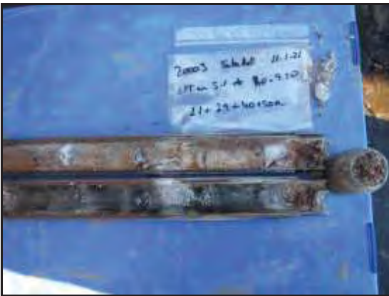
Foto 7: Sondeig S-1, SPT a 8,0 metres.
