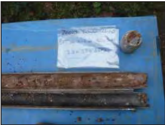
Foto 24: Sondeig S-3, SPT a 9,0 metres.
